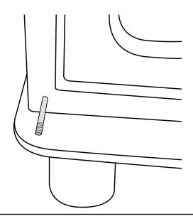
Slide the Smoke Control spacer onto the air vent control rod.
