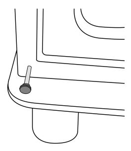
The Air Control on appliances modified for Smoke Control cannot shut down completely.
