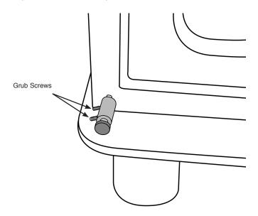
Tighten the 2 grub screws using the 2mm allen key supplied.
