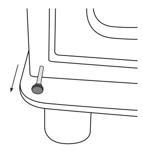
Unscrew the knob from the end of the air vent control rod.
