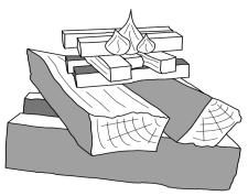
Close the door of the appliance and open both air controls; see the diagram over page. When the flames are stable and the chimney warm close the ignition vent control, or overheating can occur, which is not cover by the warranty.
