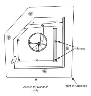
Tighten the screws to secure the Smoke Control Stop.
