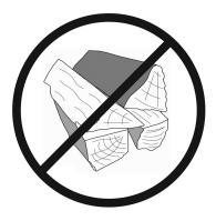
Compact stacking will make the wood burn slower as wood can only reach the outside of the fire. This will cause the fire to smoulder and produce smoke.
