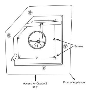
Slide the cutouts on the Smoke Control Stop onto the screws, ensuring that the tab is towards the back of the appliance and facing down.
